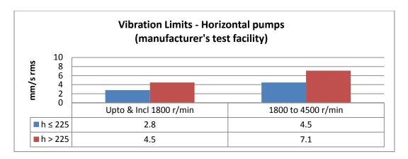
Differentiated on pump centreline height and pump speed
