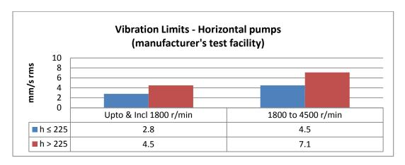
Differentiated on pump centreline height and pump speed
